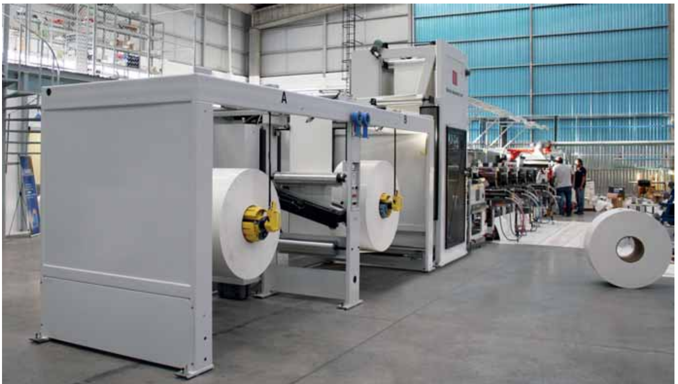
Martin Automatic MBX butt splicer on OMET's Varyflex press
